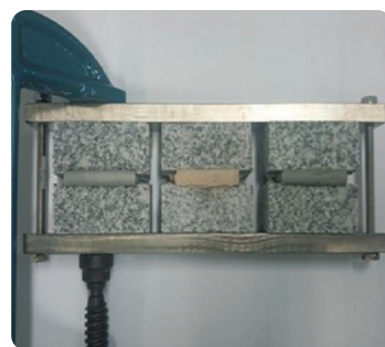
Staining test (ASTM C 1248)
